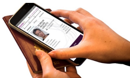
Figure 9: NFC scanning of identity document via mobile phone (from ReadID promo picture).
